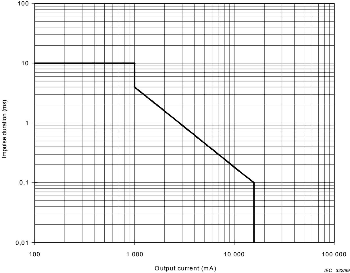
NOTE The equation of the line relating impulse duration (ms) to output current (mA) for 1 000 mA < output current < 15 700 mA, is given by  $\text{impulse duration} = 41,885 \times 10^3 \times (\text{output current})^{-1,34}$
